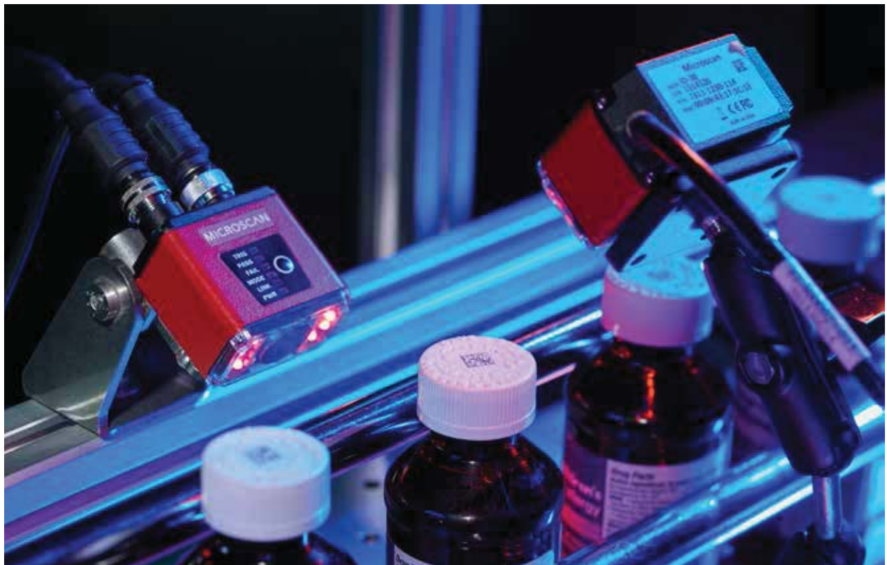
MicroHAWK ID-30 cameras scan codes placed on medicine bottle caps
